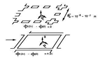
Figure 3: The penetration of magnetic field into a super conductor of type I
